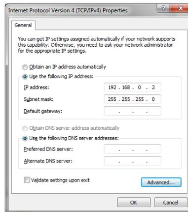
Figure 304. Internet Protocol (TCP/IPv4) Properties Screen
