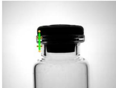
Figure 214. Edge Tool at the Left Side of the vial
