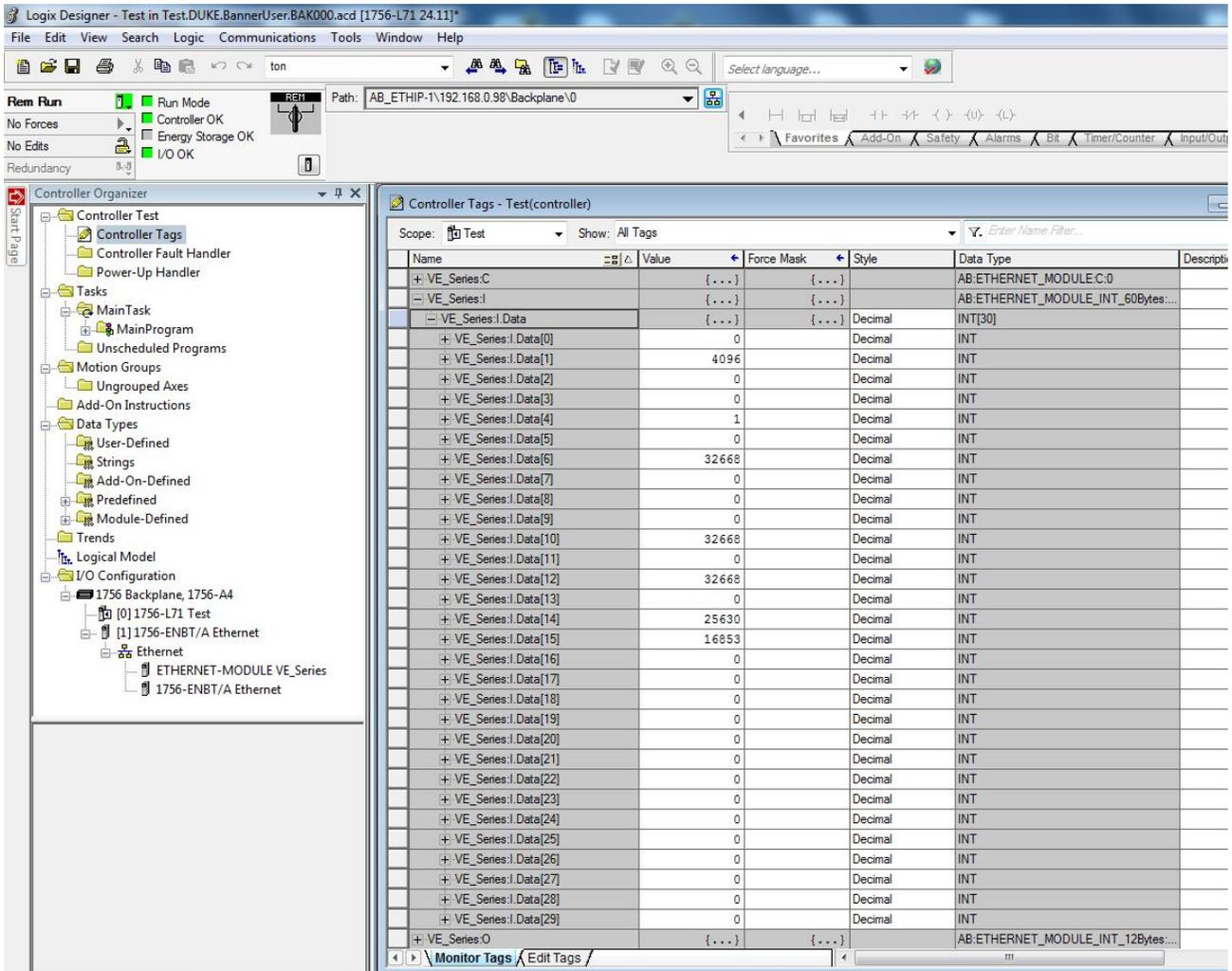
The VE Series camera memory map expanded. I = Inputs to PLC (outputs from the device).
