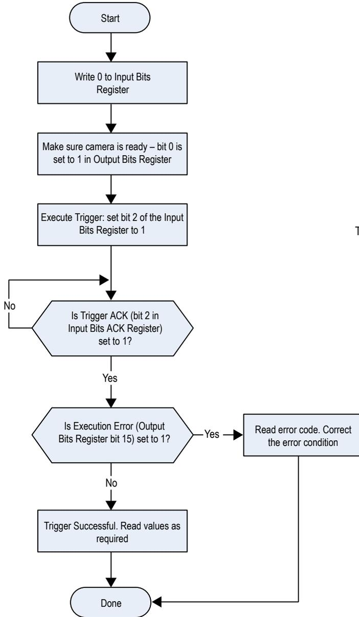
Figure 335. Trigger—Modbus/TCP, EtherNet/IP, PCCC
