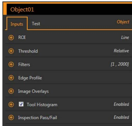
Figure 244. Object Tool—Input Parameters
