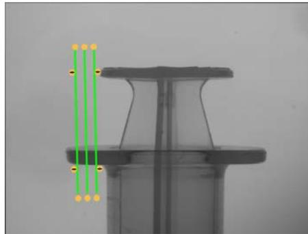
Figure 175. ROI Over the Top of the Barrel
