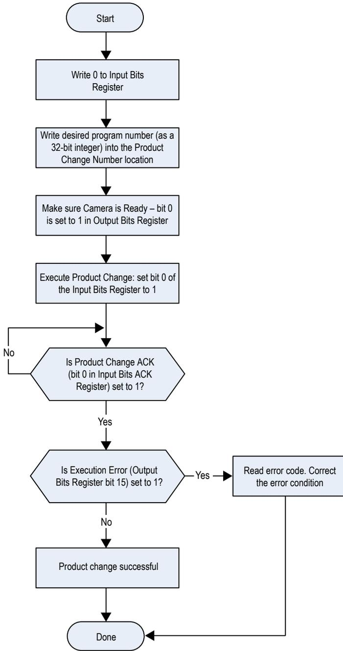
Figure 346. Product Change—Modbus/TCP, EtherNet/IP, PCCC
