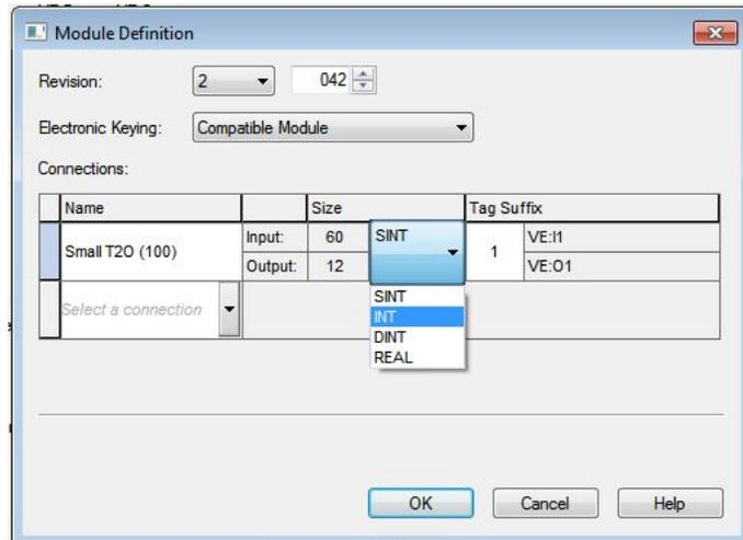
Figure 322. Module Definition—Data Type
