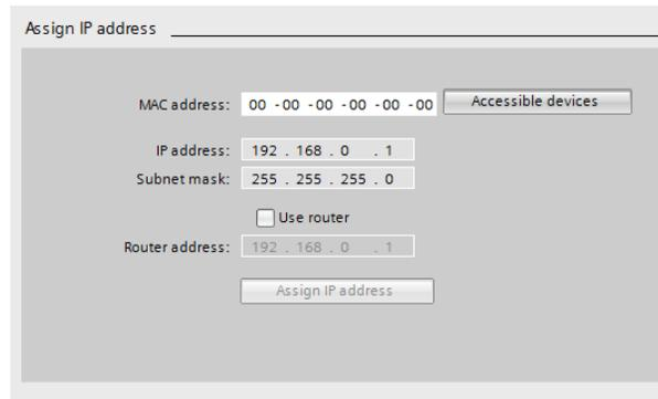
Figure 374. Assign IP Address—Accessible Devices
