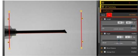
Figure 191. Bad Part—Deformed Needle
