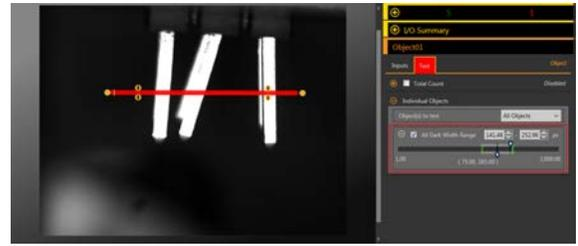
Figure 263. Bad Part—Bent Pin
