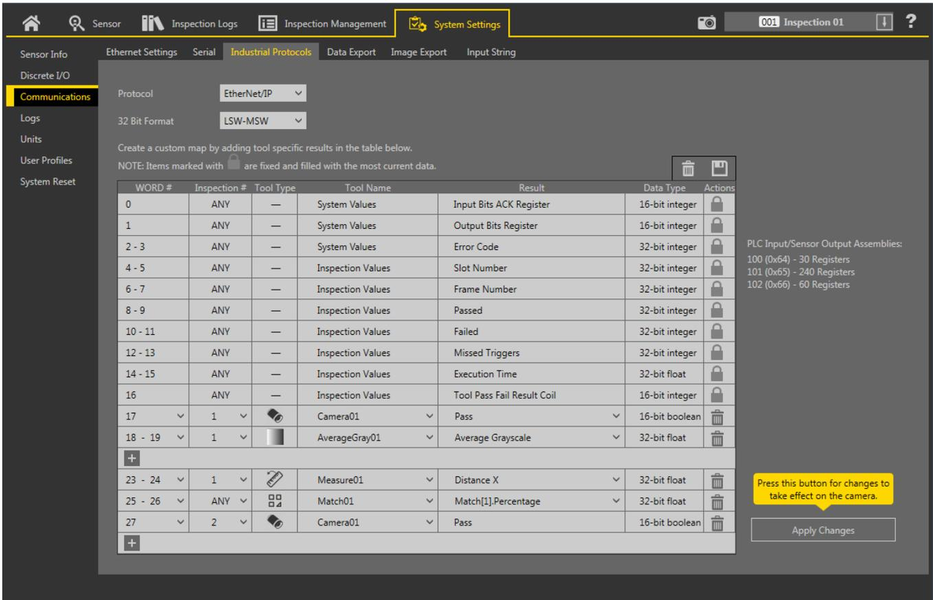
Figure 311. Industrial Protocols Tab—EtherNet/IP
