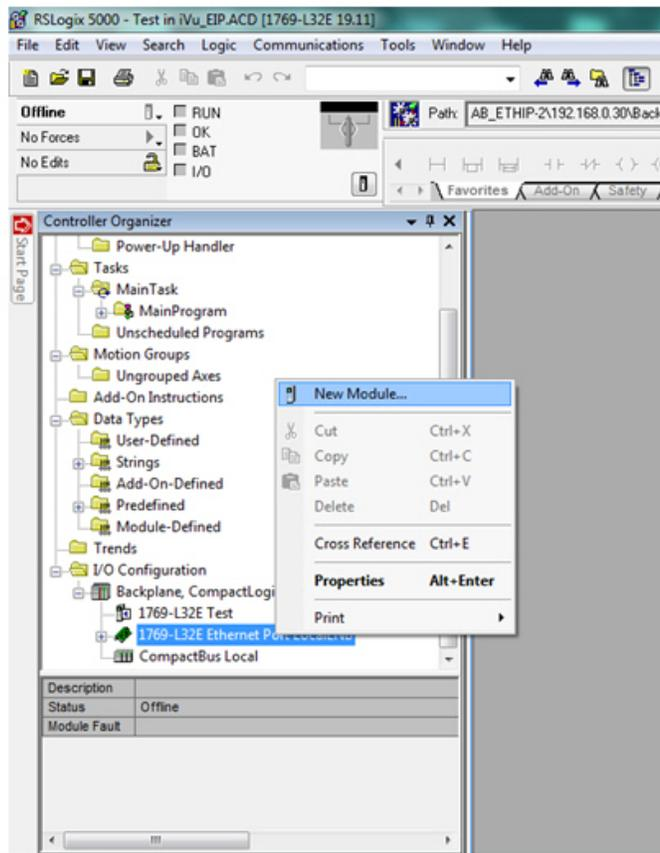
Figure 324. Add Ethernet Module
