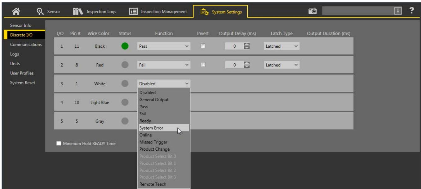
Figure 38. Discrete I/O
