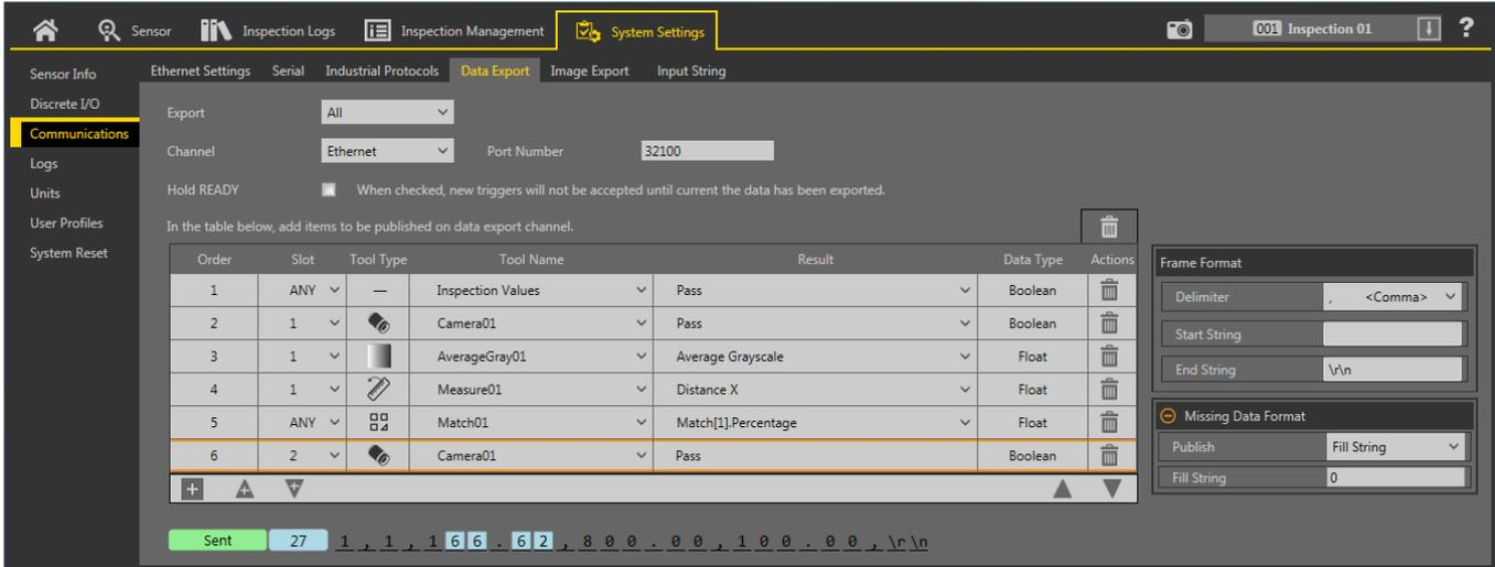
On the **Data Export** tab, set the data export parameters, including which results to export, which channel to use, and the port number to use. Note that the port number cannot be the same as any other port in use.
