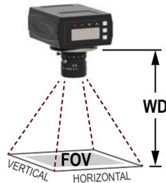
Figure 395. Working Distance and Field of View
