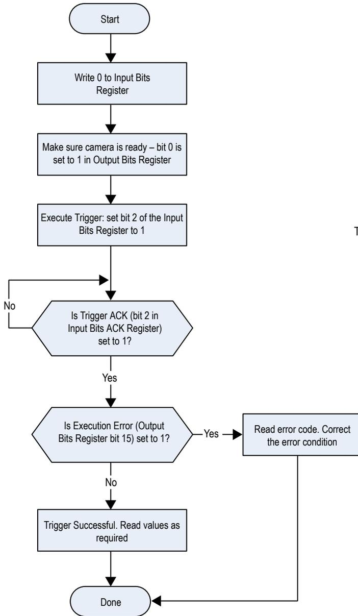
Figure 342. Trigger—Modbus/TCP, EtherNet/IP, PCCC
