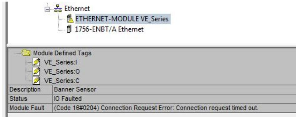
Figure 332. ERROR: VE Series camera Not Powered Up or Ethernet Cable Not Attached
