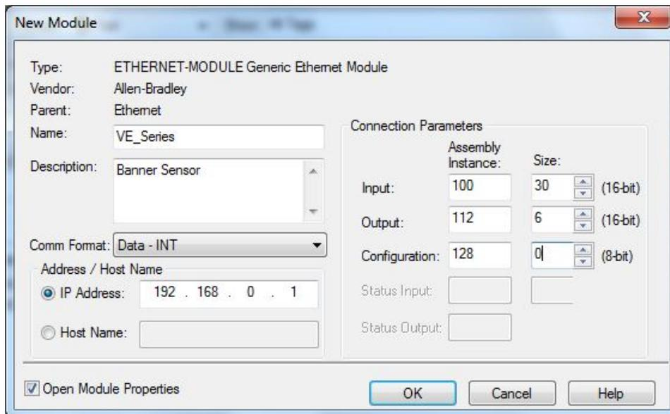
Figure 326. Example: PLC Input Assembly Instance 0x64 (100), PLC Output Assembly Instance 0x70 (112)
