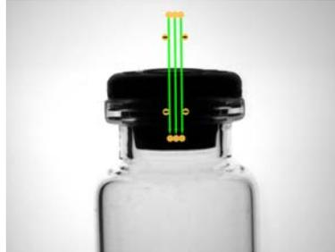
Figure 213. Edge Tool at the Top of the Stopper
