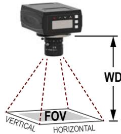
Figure 397. Working Distance and Field of View
