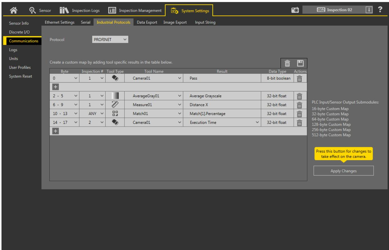
Figure 359. Industrial Protocols Tab—PROFINET
