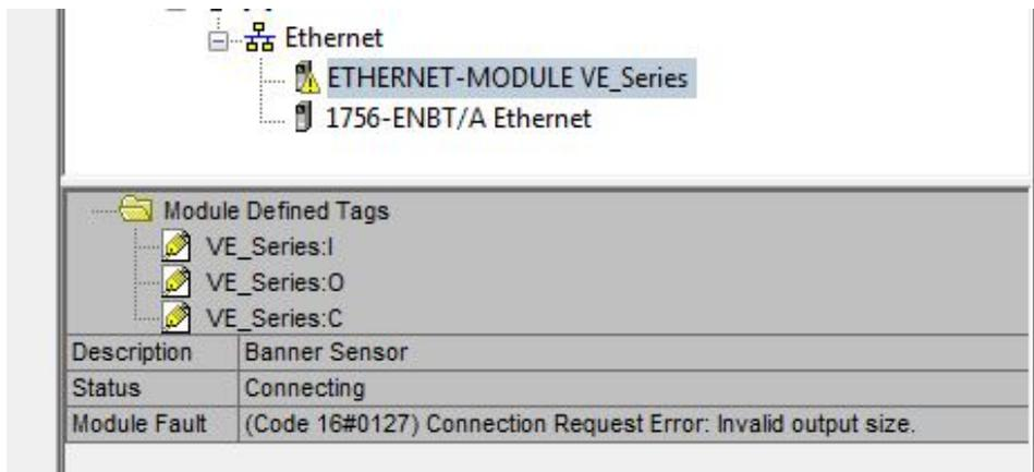
Figure 331. ERROR: Assembly Instance Number and/or Size Incorrect
