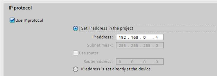
Figure 376. Siemens TIA Portal (v13): IP Protocol Options
