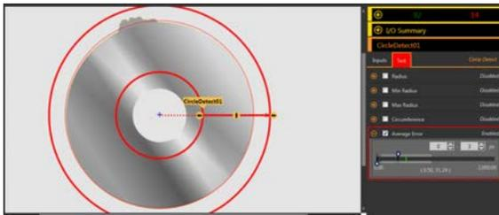
Figure 155. Bad Part—Flashing
