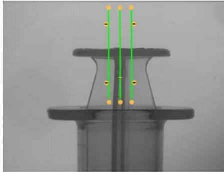
Figure 174. ROI Over the Top of the Plunger
