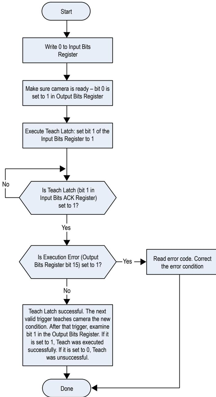
Figure 307. TEACH—Modbus/TCP, EtherNet/IP, PCCC
