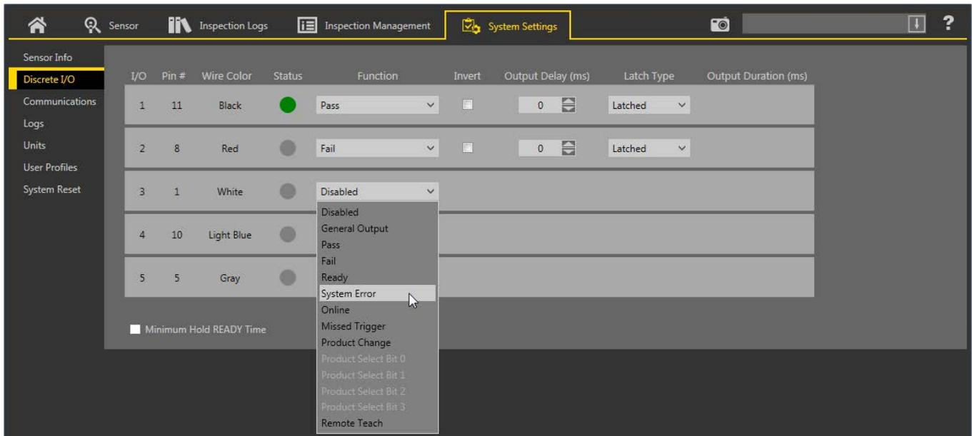
Figure 15. Discrete I/O
