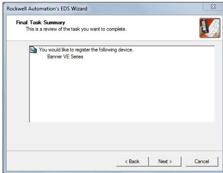
Figure 317. Register the EDS File
