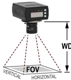
Figure 396. Working Distance and Field of View
