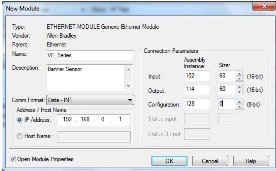
Figure 328. PLC Input Assembly (102), PLC Output Assembly (114)
