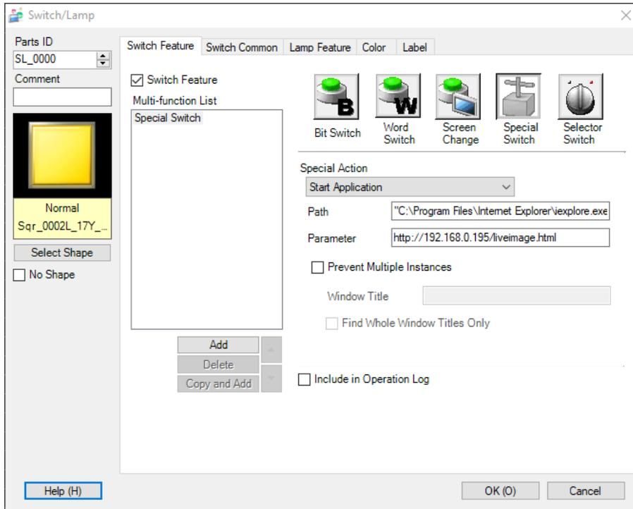
Figure 391. GP Pro-EX Software Special Switch part used to Start Application, pointed to web browser with IP address Parameter
