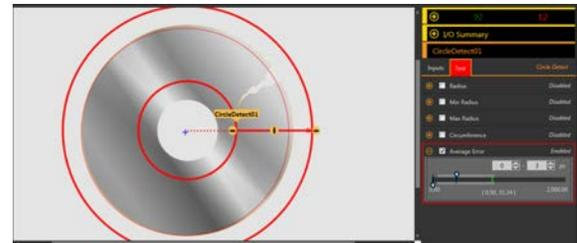
Figure 156. Bad Part—Crack
