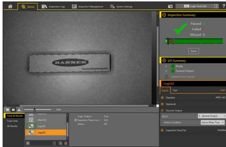
Figure 297. I/O Summary—Small Box Passes with Output
