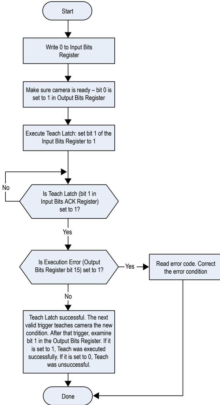
Figure 337. TEACH—Modbus/TCP, EtherNet/IP, PCCC
