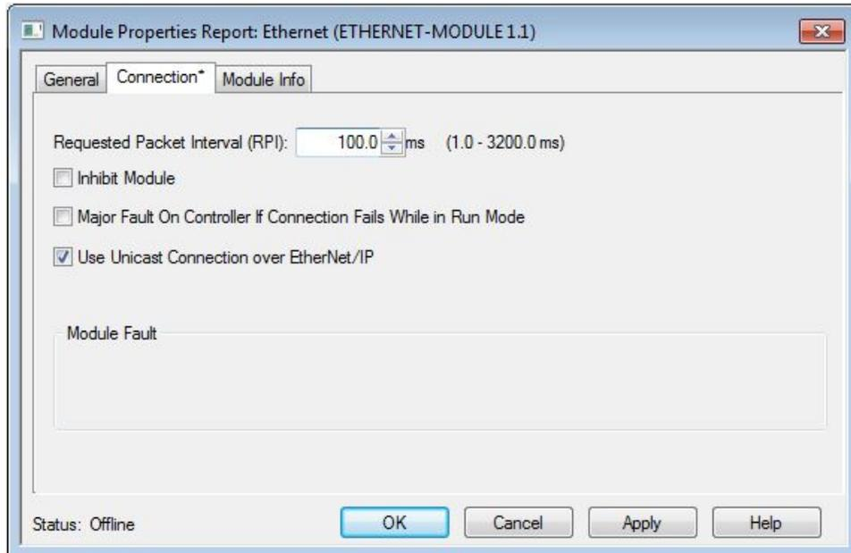
Figure 329. Select or clear the Unicast Connection checkbox as desired
