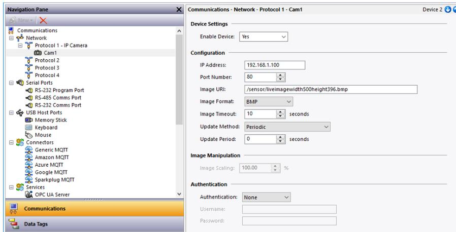
Figure 392. RedLion IP Camera protocol selection
