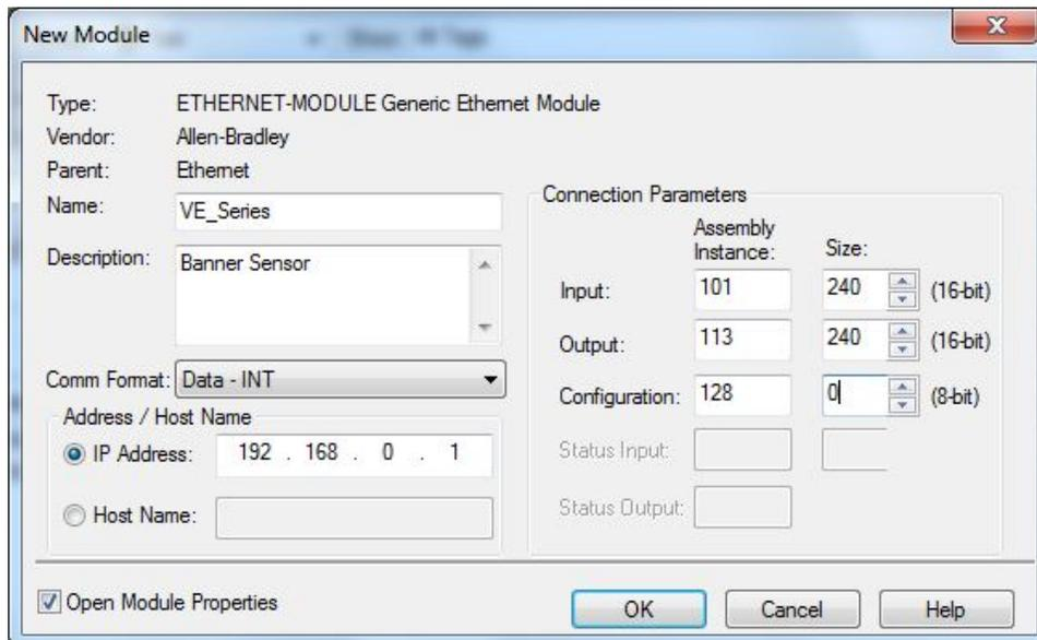
Figure 327. Example: PLC Input Assembly Instance 0x65 (101), PLC Output Assembly Instance 0x71 (113)
