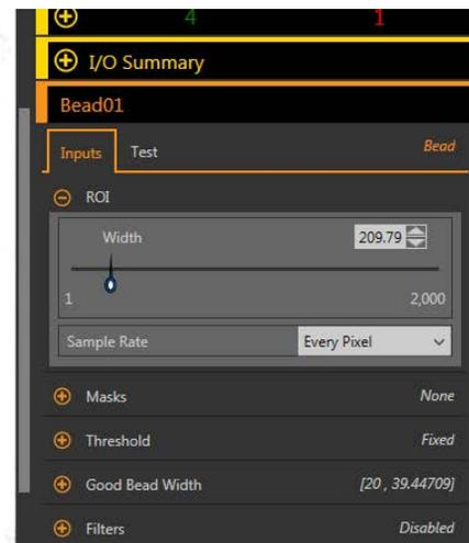
8. Use the **Good Bead Width** parameter under **Characteristics** to define the good bead width.
