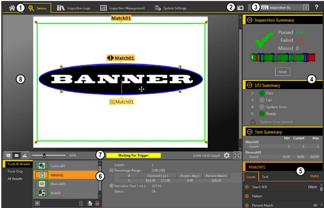
1. Screens—**Home, Sensor, Inspection Logs, Inspection Management, System Settings**
