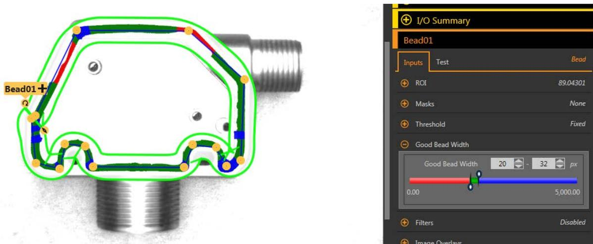
Figure 102. Good, Narrow, and Wide Adhesive Widths
