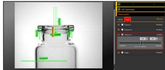
Figure 220. Bad Part—Missing Stopper
