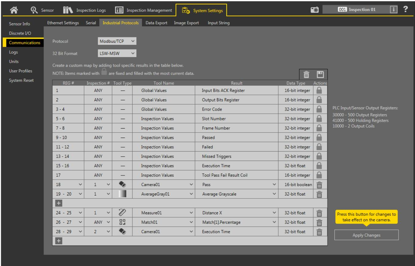
Figure 341. Industrial Protocols Tab—Modbus/TCP
