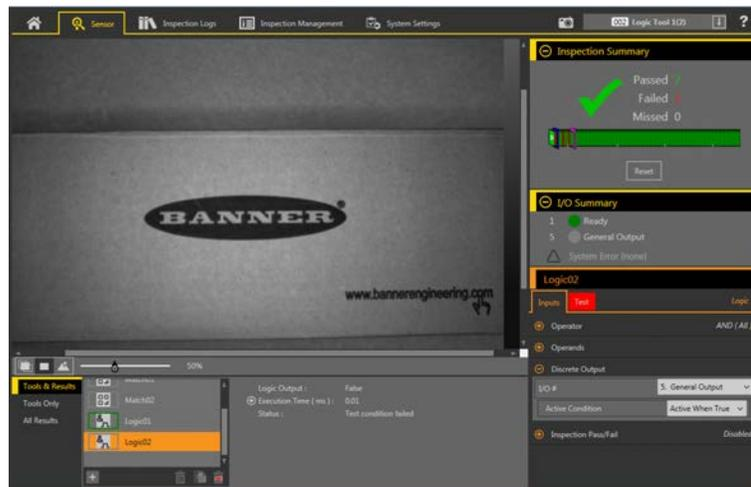
Figure 298. I/O Summary—Large Box Passes with no Output
