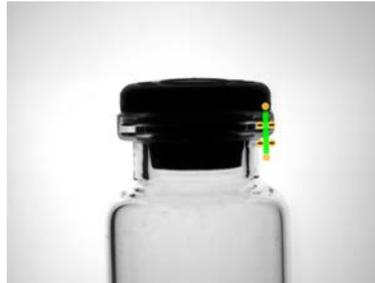
Figure 215. Edge Tool at the Right Side of the vial
