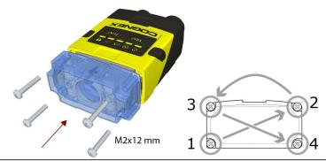
(i) Note: The rib in the front cover must be oriented to the top side.
