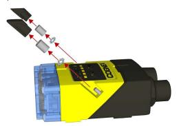
3. Detach the main module and the I/O connector module by firmly pulling them apart.
