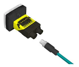
2. Connect the Ethernet cable's RJ-45 connector to a switch/router or PC, as applicable.
