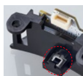
Photodiode and correction circuit within the lighting
