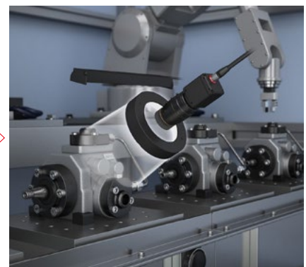
Appearance inspection of metal processed surfaces after settings changeover to Program 0002
