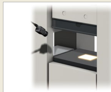
NG product (workpiece displaced)
